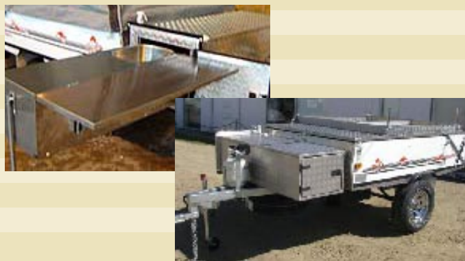
The Stainless Steel Kitchen Rolls Out of the Aluminium Box Mounted on the Drawbar.
