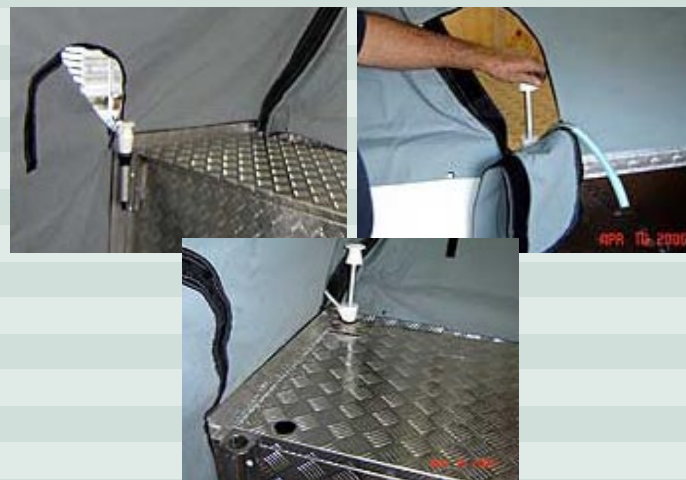
The Kitchen with a 16 Gallon Water Tank with Hand Pump
